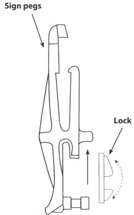
(For hanging main sign panel beneath cross-arm, and, for attaching side of main sign panel to upright post to prevent swinging)
