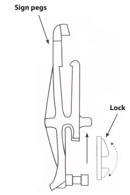
(For hanging main sign panel beneath cross-arm, and, for attaching side of main sign panel to upright post to prevent swinging)
